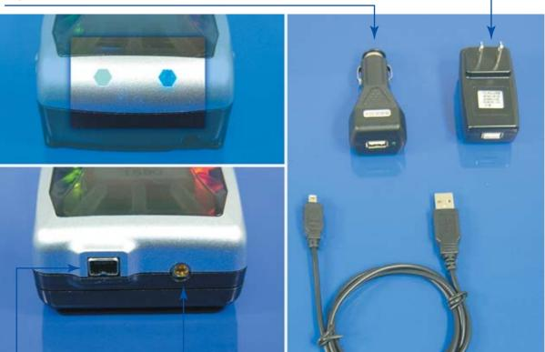
Mini-1394 female connector for power in and GPS signal out
